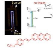
Conductive and emissive: Organic transistors made from a simple styrylanthracene derivative (see scheme) have high charge mobility and high luminescence quantum yields. These properties are attributed to the lack of singlet fission, and challenge the idea that the efficient  $\pi$ interactions required for high mobility always lead to quenching of emission. The transistors emit blue electroluminescence and are stable during operation and storage.
